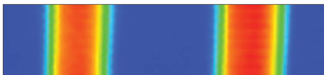
Figure 3. A single un-processed scan across the ATR test target covering a 100 micron width and showing absorption at 1726\text{ cm}^{-1} . The air gaps show as deep blue (zero absorption), whereas the plastic regions in contact with the crystal show as red (0.21 absorbance). There are scan lines from each of the 16 detector elements in this image.
